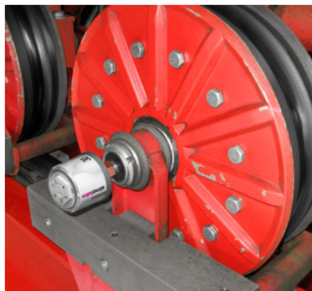
The guide rollers of a mountain railway are supplied with the necessary lubricant.
