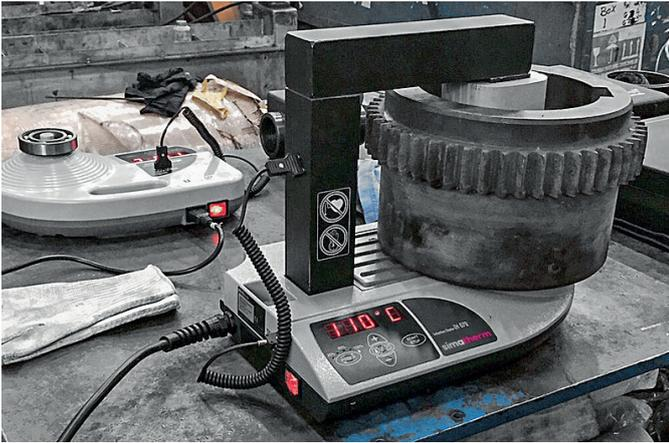
The simatherm induction heaters VOLCANO IH 025 and IH 070 with two differently sized workpieces: the model IH 070 (in the front) heats a gearwheel sleeve to the specified installation temperature.
