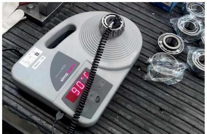
The portable VOLCANO IH 025 is used for the installation of gear shafts. For this purpose, a tapered roller bearing is heated to the desired temperature using the temperature monitoring system.
