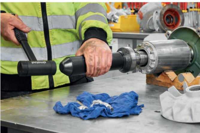
The Fitting Tool FT 33 ensures that the mounting force is evenly distributed across the inner and outer rings of the bearing and therefore does not stress the rolling elements.
