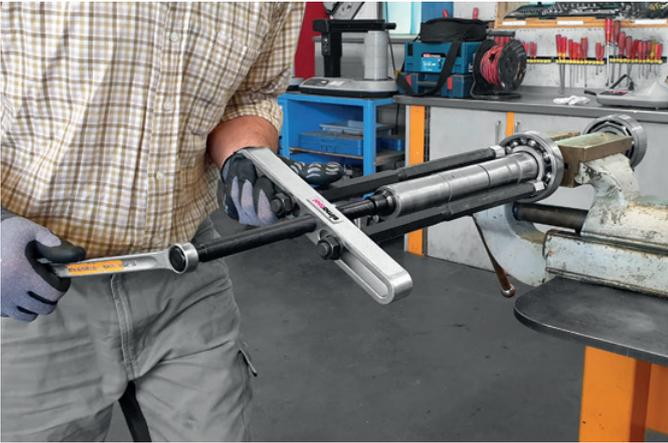
With the aid of extensions, the BP 160 dismounting tool kit also makes it possible to dismount hard-to-reach bearings easily and professionally.
