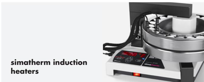
The best way to avoid unwanted stresses when assembling interference-fit parts is to heat the outer part just enough to produce a temporary clearance. simatherm induction heaters allow this to be done precisely, evenly, quickly and efficiently. Other methods of heating are slower, less controlled and can cause more harm than good to bearings.
