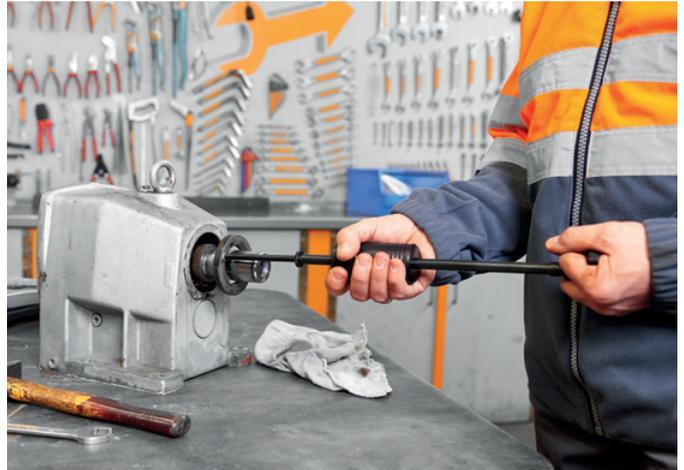
Knowhow: using a Seal Puller SP 50 to remove a radial seal from a gearbox without damaging the housing or shaft.
